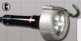
XP99 Hazardous Location Spot Light - Great for the Class 1, Division 1, Group D hazardous locations, this unit comes standard with a 50 watt, 12-volt sealed beam lamp. The lamp produces 100,000-candle power and is excellent for inspecting large vessels or vats. The outer shell is made of a corrosion resistant, non-sparking metal and comes with rotating hook.
